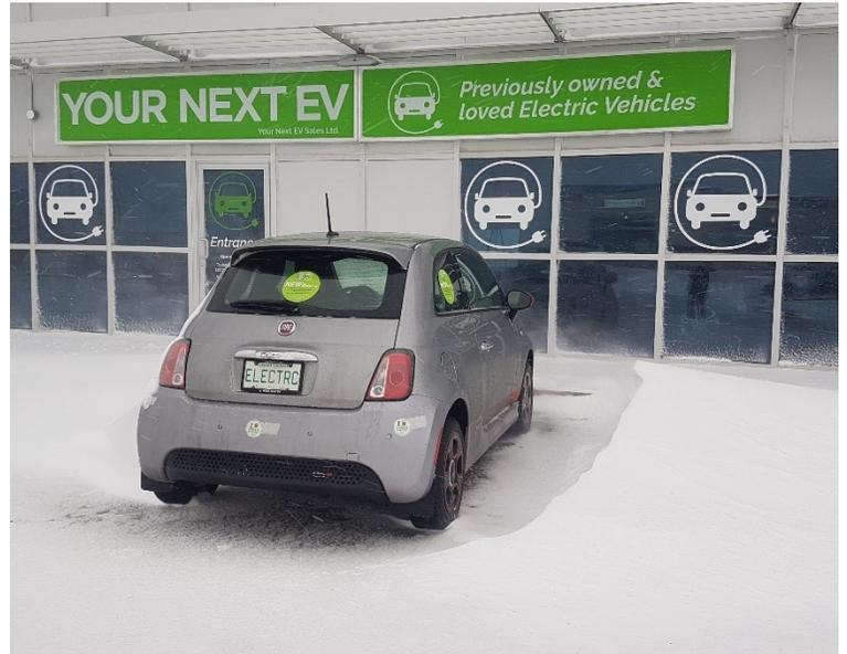
This car has a 24 kWh battery with an EPA-rated range of 135 km. Its practical range in summer is about 120 km, meaning that I have a few kilometers of range left when I get home. This summer range is under urban driving conditions or with some highway driving at 95 km/hr or so. Faster speeds will reduce the range as will driving at night with the headlights on. This practical range assumes some use of air conditioning.
